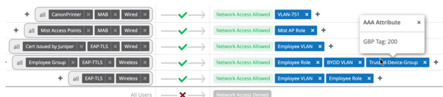
Figure 7: Enforced policies for VLANs, group-based policies, and user roles are easily visible
